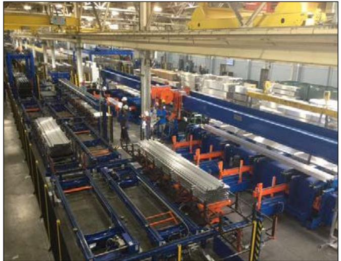
Figure 1. Automated profile stacking system in the foreground with the newly installed lineal packing system behind.
