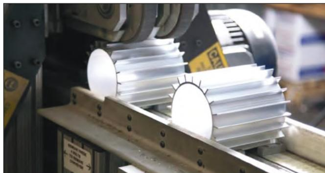
Figure 2. Dual head deburring of 6063 sump housings.
