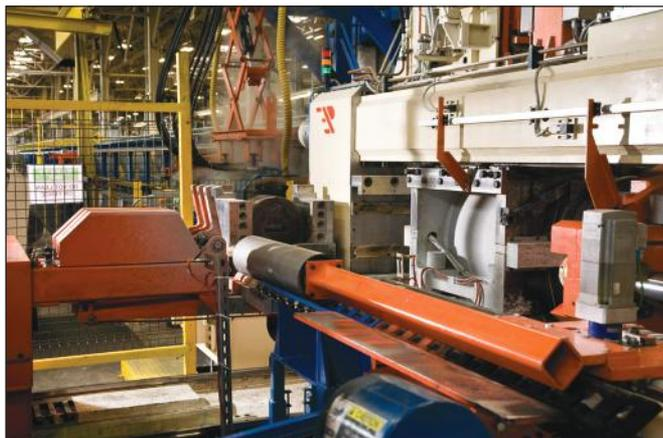
Figure 5. Loading of billet into the 8 inch, front loading press.
