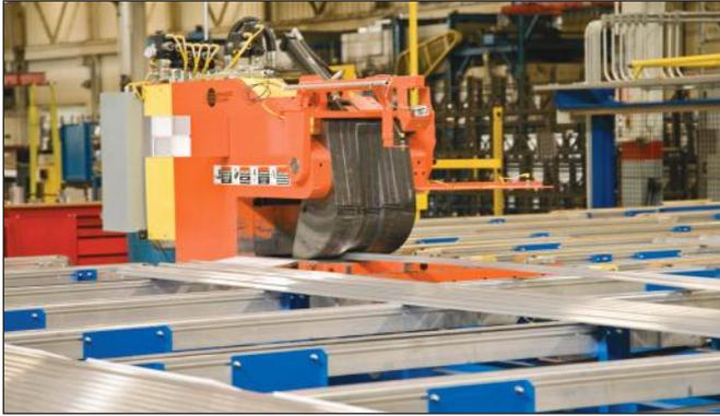
Figure 8. Stretcher (75 ton) installed for the 8 inch press line.
