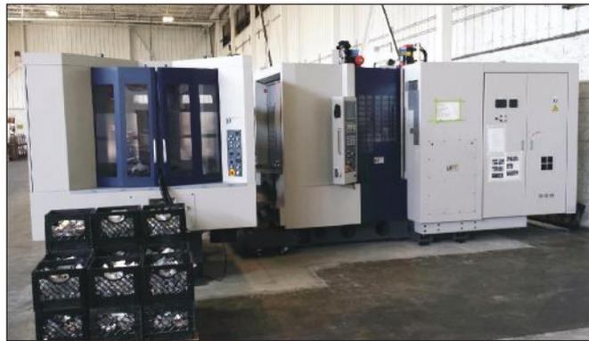
Figure 3. Newly acquired Kiwa KH-45 six pallet horizontal machining center.
